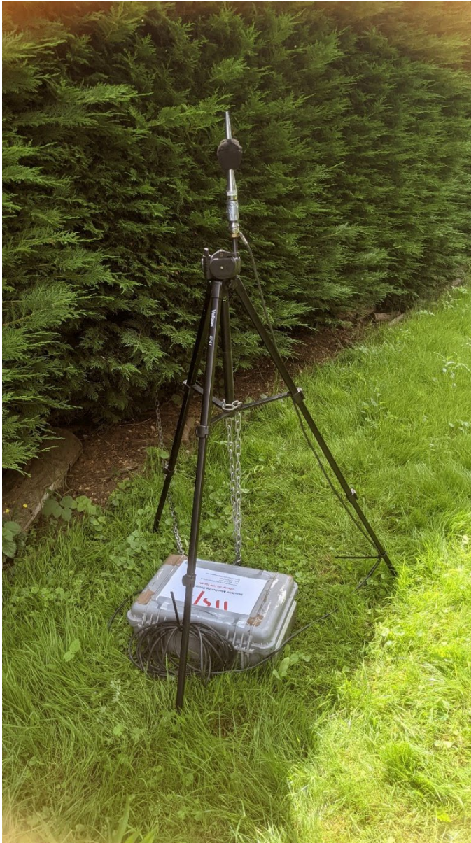
Figure 2.1 – Site photograph of noise monitor at MP1
